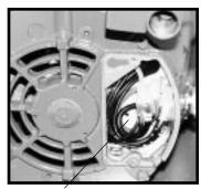
Motor wires exposed
