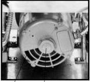
Vent slots Shaft cover Figure 3.2C
