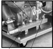
Supply manifold Figure 6.1H Pressure switch line
