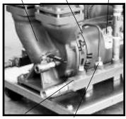
Supply Manifold Pump seal Figure 6.1A cooling line
